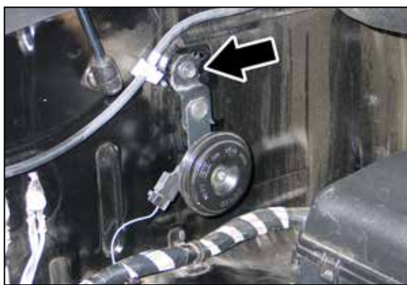
13. On vehicles equipped with a security system horn, remove the bolt which secures the horn to the inner fender.
