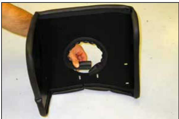
10. Install the small edge trim into the hole of the heat shield as shown.
