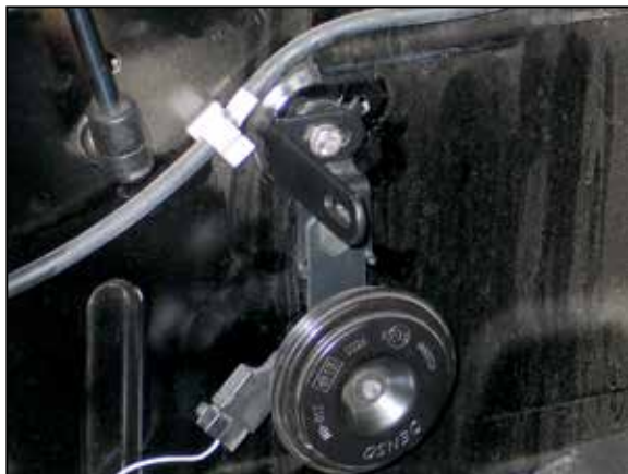
14. Install the small "L" bracket (070742) onto the inner fender using the hardware provided as shown.
