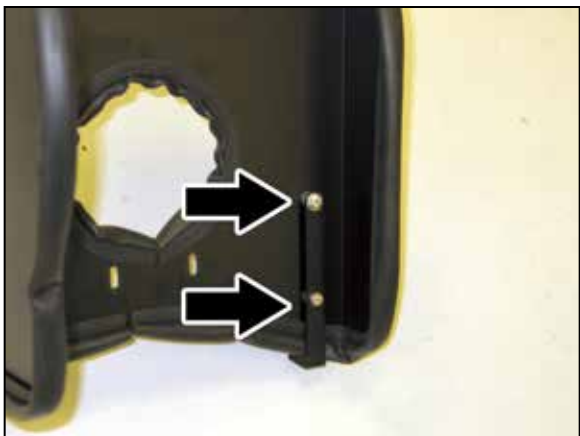
11. Install the large "L" (070902) bracket onto the heat shield as shown using the provided spacers and hardware.
