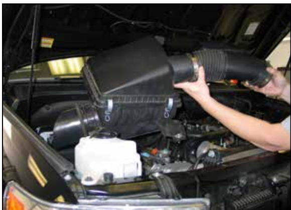
8. Remove the complete stock intake assembly from the vehicle as shown.
