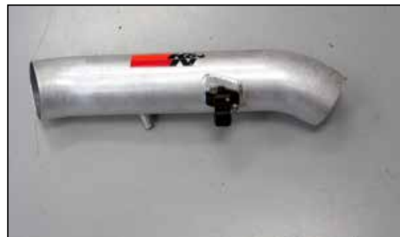
20. Install the mass air sensor into the K&N® intake tube using the hardware provided.
