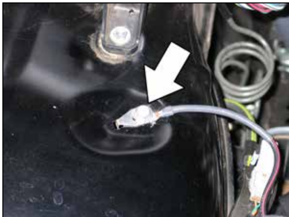
15. Remove the bolt which secures the ground strap to the inner fender.
