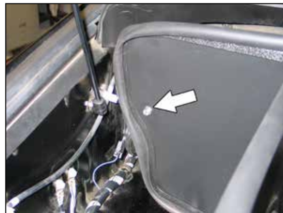
18. Secure the rear heat shield bracket installed during step #14 to the heat shield with the provided spacer and hardware.
