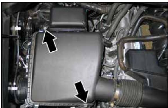
7. Loosen the two bolts which secure the air box to the inner fender.
