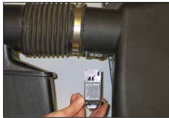
19. Remove the two bolts which secure the mass air sensor into the stock air filter housing and then remove the mass air sensor as shown.
