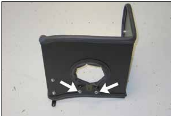
14a. Install the tube mounting bracket on the heat shield as shown using the provided hardware.
